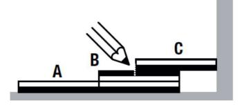
Finally, install the cut Tile B in the space between the wall and Tile A.
